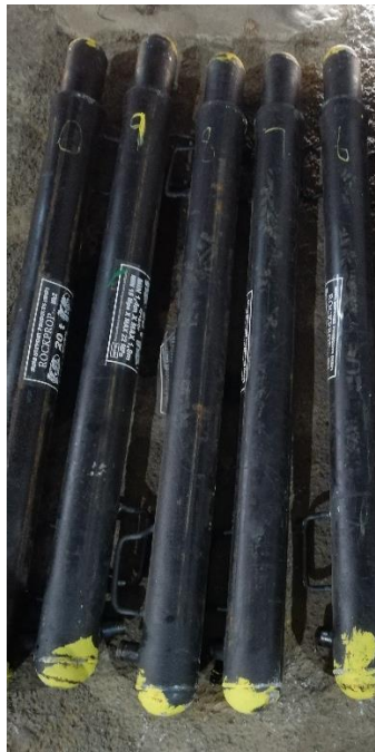
Figure 1: MK2 Rocprops before dynamic test
