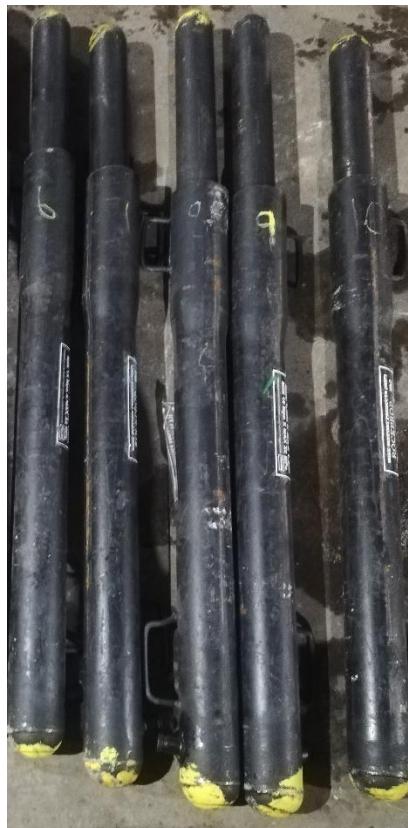
Figure 2: MK2 Rocprops after dynamic test
