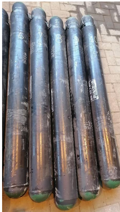
Figure 1: Five MK1 Rocprops before dynamic test
