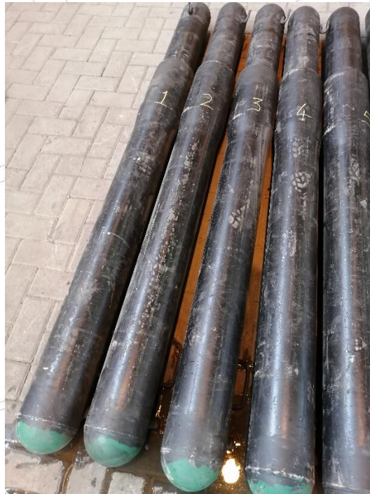
Figure 2: Five MK1 Rocprops after static testing
